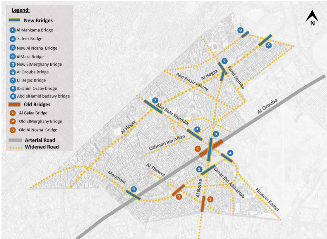
Figure 27: Map of new bridges and expanded roads of Heliopolis after the development. Source: Illustration by the author, the base map is from Google Earth/Maps 2022
