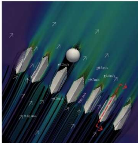
b) Streamline wind flow diagram (x, y plan, h=1.2m) at Huta Sialagan
