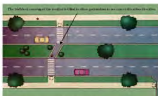
Figure 4.2 - A model of midblock crossing. Source: Road Elements Coordination Standards Manual
