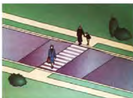
Figure 4.3- A model of a raised floors. Source: Road Elements Coordination Standards Manual
