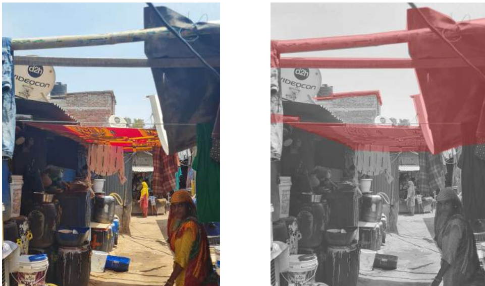
(Figure 26)- Left image showing the typical internal street of the slum and right one highlighted the inflammable materials in red used like bamboo, clothes and plastic sheets (Source: author).
