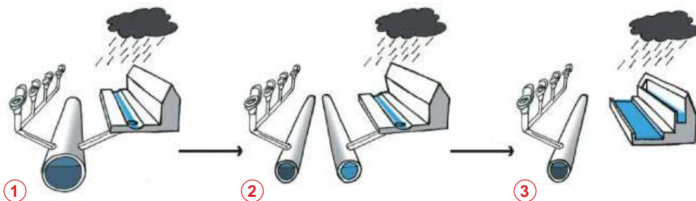
Figure 80: Dynamics between sewage water and rainwater networks. Number 1 : Both liquids mix in a main pie. Number 2: every liquid has its own network, which allows recycling. Number 3: waste water has pipes and the city becomes a retention point for storm water. Source: http://marcovermeulen.eu/themes/11/waterindestad/46/watersquares/english/
