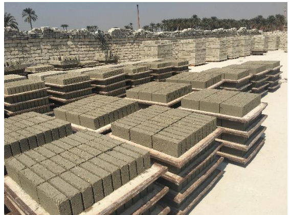
Figure 14: Front; Cement bricks stalked for sun drying, behind; Dried bricks ready for transfer. (Source: Author)
