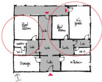
Figure 6.36: Analytical sketch showing the double attached apartments in one house
