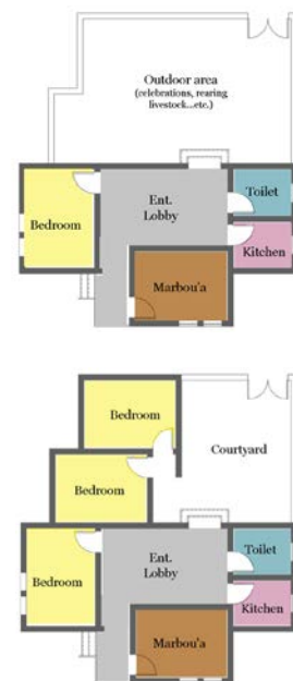
Figure 6.45: Above: Floor plan for the proposed future governmental prototype. Below: The suggested future expansions (Source: General Administration for Project, NWCDA, Maṭrūh)
