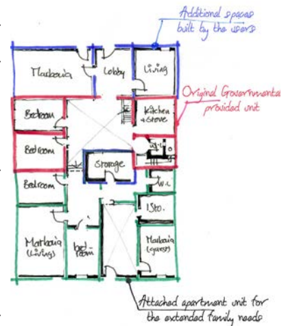
Figure 6.14: Ground floor plan of sample unit with its reasoned amendments (Read: the original core house, Blue: the added spaces by users, Green: the extension added to accommodate the extended family needs)
