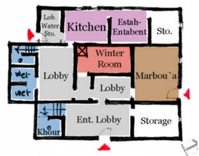
Figure 6.06: The ground floor plan of the discussed vernacular house (drawn by the researcher as observed during the fieldwork with some clarifications by its former resident)
