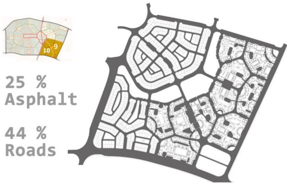
Figure 73 Percentage of roads and asphalt in neighbourhoods 9 & 10 in Al Rehab. Source: (Yousry, et al., 2005) adapted by Author
