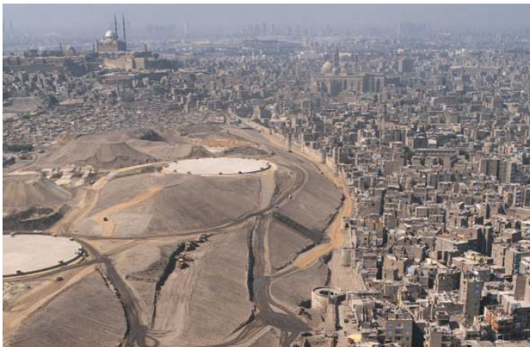
Figure 4-11: An aerial view of the project site shows the topography of the Azhar Park after master grading. The photo also shows one of the three water tanks, being integrated into the emerging new park topography. On the edge of the site is the uncovered Ayyubid city wall. To the right, the Darb al-Ahmar district appears (Source: AKTC, 2012).
