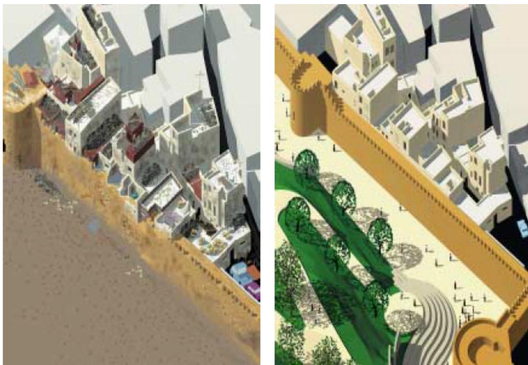
Figure 4-14: Improvements of old houses along the historic wall. Left: schematic rendering of existing conditions in Atfet Assad. Right: schematic rendering of the integrated pilot project, showing improved conditions after selective removal of encroachments on top of the wall. Physical and social rehabilitation of housing goes hand in hand with the wall restoration (Source: AKTC, 2012).
